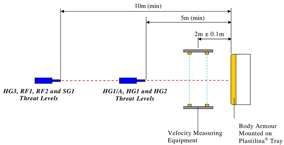
**FIGURE 3:** Typical Test Apparatus for Ballistic Testing
