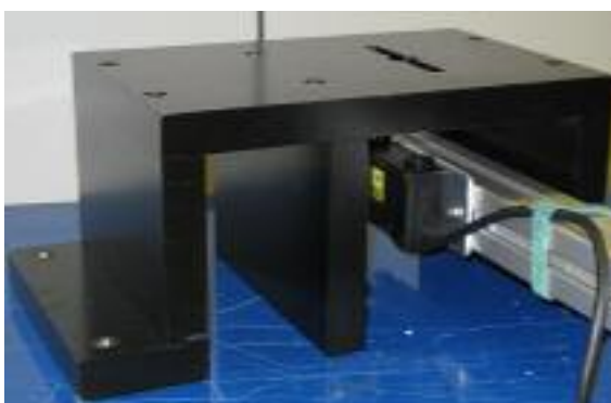
Figure 4 Soft Tissue Protector Test Anvil
