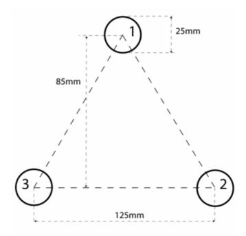
FIGURE 6: Small Size Front Panel
