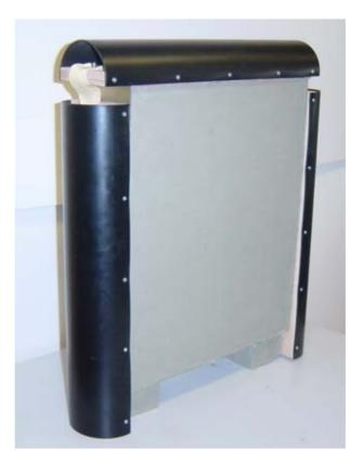
Figure 2 Ballistic Shoulders Positioned on Test Block
