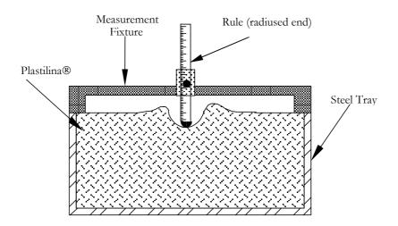
FIGURE 5: Method of Measuring Back-face Signature
