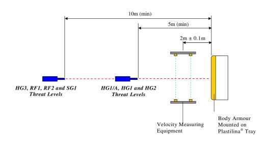
FIGURE 3: Typical Test Apparatus for Ballistic Testing
