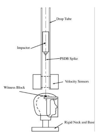
FIGURE 8 Penetration Test
