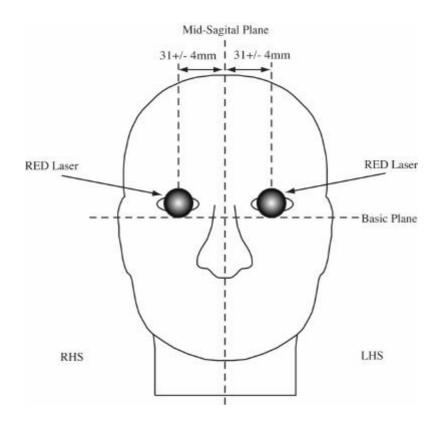
FIGURE 10 Example Headform with Laser
