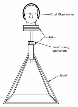
FIGURE 5 Test Mount for Acoustic Test
