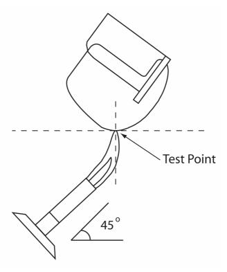
FIGURE 6 Flame Test
