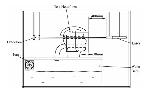
FIGURE 13 Visor Mist Test
