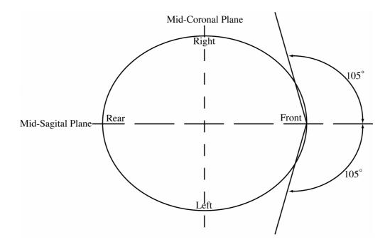
FIGURE 4 Peripheral Vision - Sidewards
