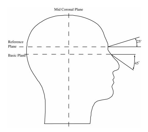
FIGURE 3 Peripheral Vision - Forwards
