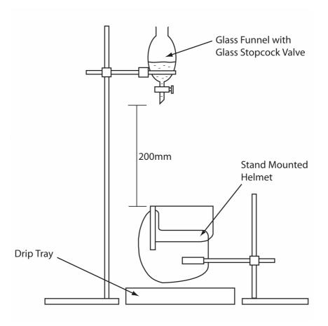
FIGURE 16 Visor Solvent Test
