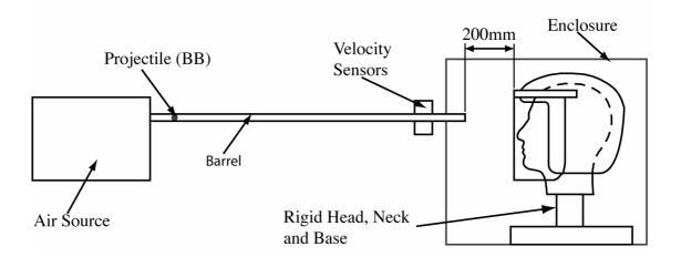
FIGURE 15 Visor Pellet Test
