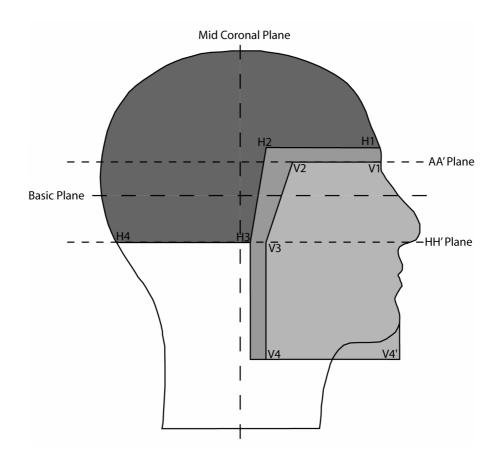
FIGURE 2 Coverage of Helmet Body and Visor
