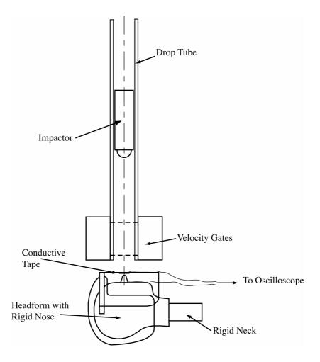
FIGURE 14 Visor Impact Test
