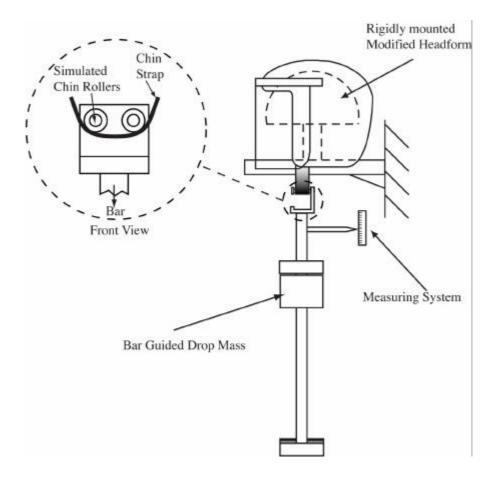
FIGURE 7 Retention Strength Test
