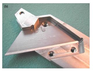
Figure 6: (a) Test blade being inserted into the pivot arm; (b) test blade located in pivot arm notches (clamping plate removed)
