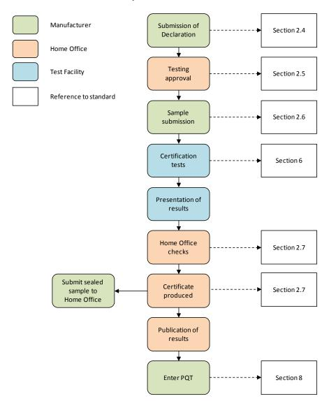
Figure 1: Process map for certification to the 2018 Slash Resistant Materials Standard
