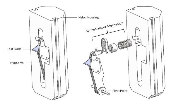
Figure 3: Slash sabot and its constituent components
