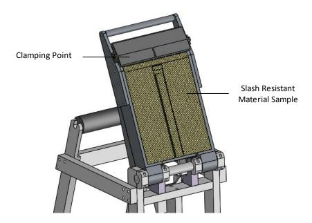
Figure 5: Mounting of test samples
