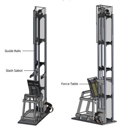
Figure 2: Home Office Slash Drop Test Assembly
