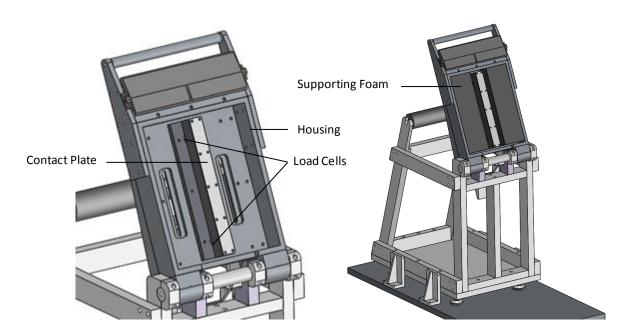
Figure 4: Force table and its constituent components
