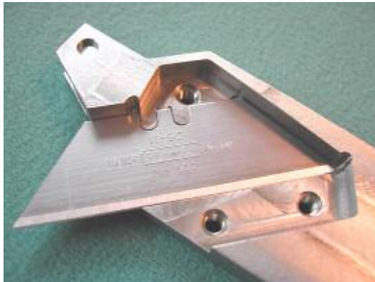
Figure 6. Test blade located in notches (clamping plate removed)
