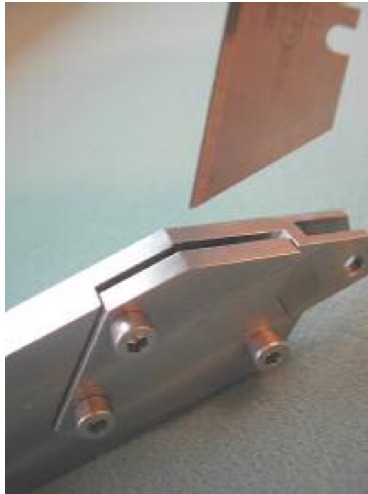
Figure 5. Test blade being inserted into the HOSDB designed supporting arm.
